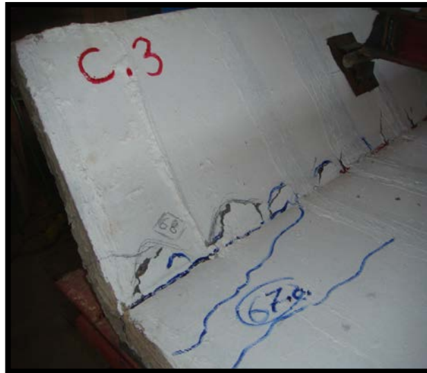
Photo 9 Final Failure in control channel C3
