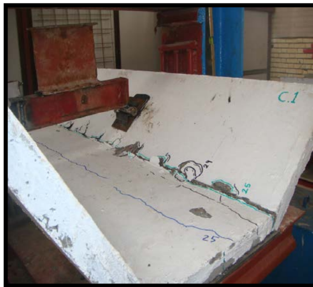
Photo 8 Final Failure in control channel C1
