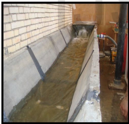
Photo 6 flume with 5 tapes from CFRP sheets
