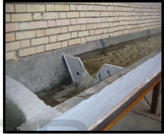
Photo 4 V-notch weir in experimental work
